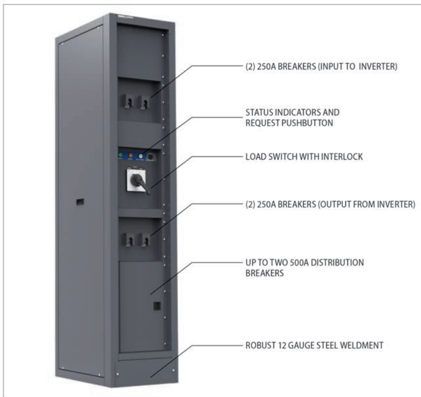
Figure 1. Manual Bypass Switch Cabinet
